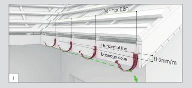
Before mounting the brackets, you should draw a drainage slope towards the place where you will place the pipes. It is preferable to make the slope of the gutter about 2 mm for each metre of its length. The distance between the hooks should not exceed 0.8 m, and the brackets at the ends should be placed 0,1 m from the edge of the roof.
