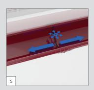
Two gutters that are to be joined should be placed on the brackets without being fixed. The distance between the edges of the gutters should be approximately 2-3 mm, as the gutters and the corners (KEB / KIB) have the property to expand and contract according to the temperature variations.
