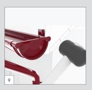
The universal stop (CU) end is fixed manually or using a rubber hammer at the end of the gutter, without using silicone because it destroys the gasket through time.
