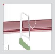
Mark a spot and use a saw and tinsnips to cut a drainage slot in the gutter, which should not be larger than the diameter of the downpipe.
