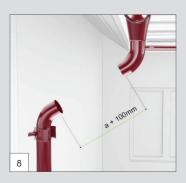
Downpipe bends 60° (CB) are mounted on the gutter outlet (RA) and down onto the downpipe (BU). They can be joined through the intermediate downpipe (PB). Measure the distance between the bends "a", add 100 mm to it, for both ends of the intermediate downpipe, each of which enter the bends by 50 mm.
