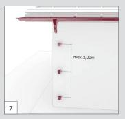
For the installation of downpipes (BU), attach the downpipe holders (BB) on the wall, one below the other, depending on the type of facade: with two side ears, central with a stud or vertical with poprivets. The maximum distance between two holders will not exceed 2 metres, while for each downpipe at least two support brackets will be used.
