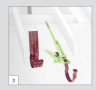
Before you mount the brackets (CJ), you should bend them so they match the angle of the roof inclination with the bending tool, according to the drainage slope.
